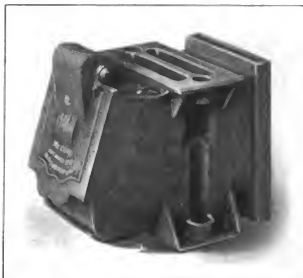
Fig. 4488. McCord Journal Box with Coil Spring Lid and Inside Dust Guard.
